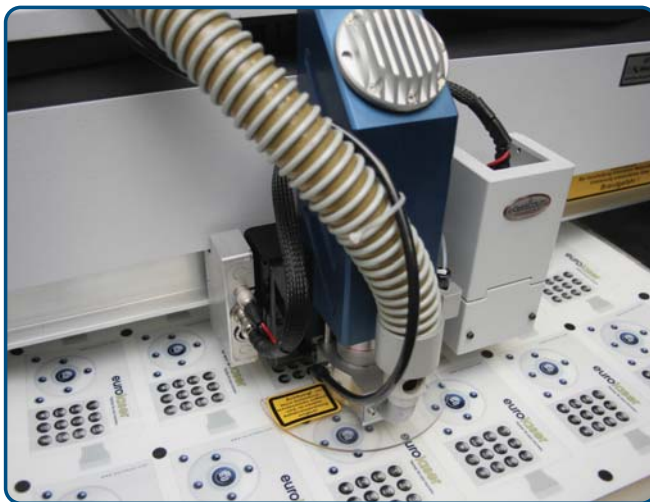
Lasercutting of printed foils by camera recognition
