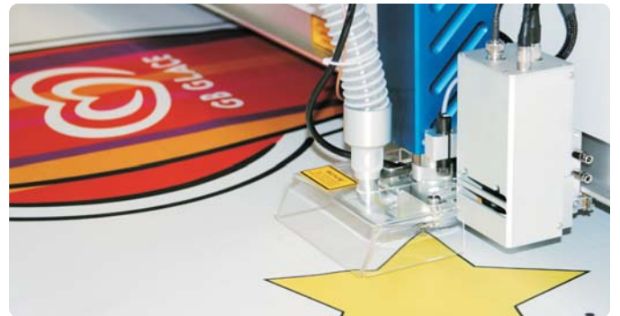
Lasercutting of printed materials by camera recognition
