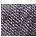
**Carbonfiber**woven, knitted or unidirectional textile structure.
