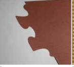
Prepreg pre-impregnated fiber. Semi-finished product of carbon or glass fibers and a non-hardened duro- or thermoplastic matrix.
